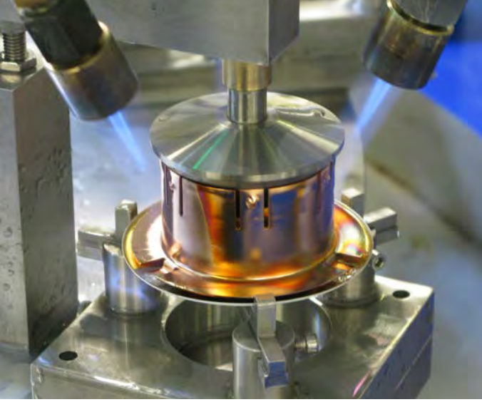
Flame heat melts fusible filler metal, bonding housing to cover plate.
