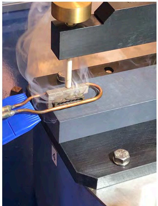
Induction coil brings silver brazing filler metal to 1305°F liquidus temperature.
