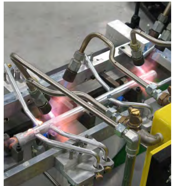
Two stations of flame heat bring the aluminum filler metal to its 1080°F liquidus temperature.
