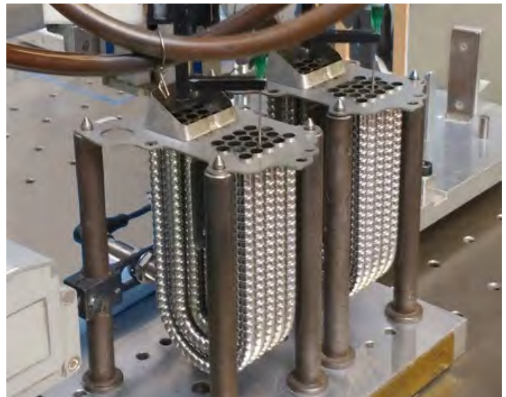
Robot-controlled, pneumatic dispenser applies multiple deposits of CNG-1630F-87X nickel braze paste to EGR assembly
