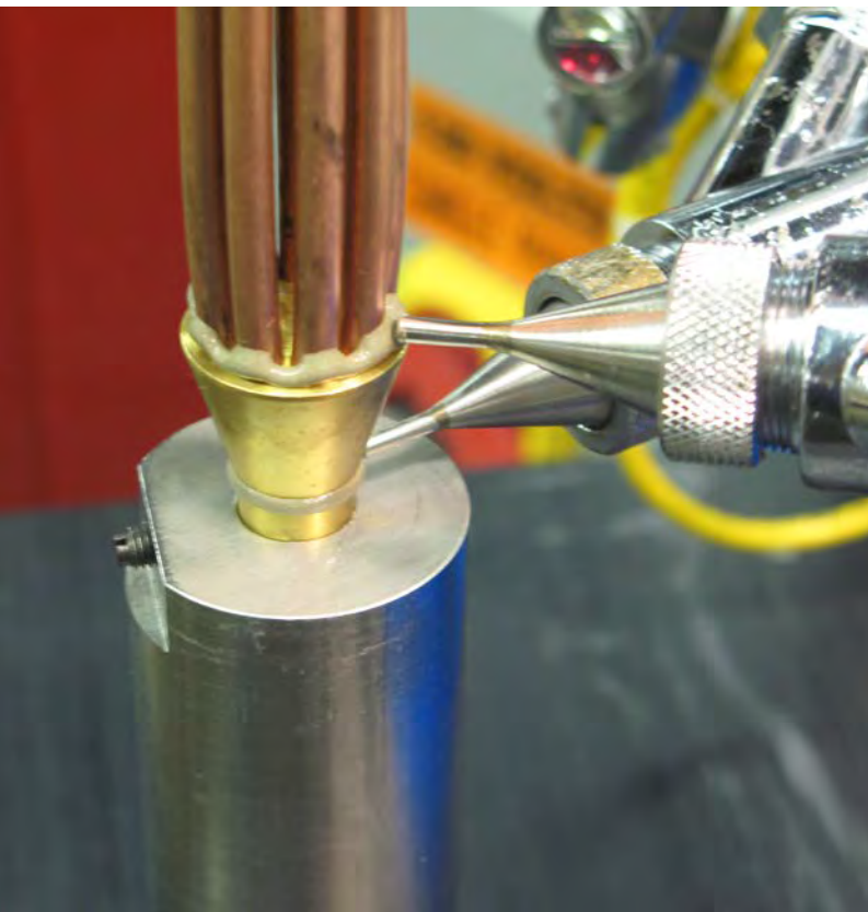
Two applicator guns dispense 360° stripes of brazing paste to all joints of distributor assembly.
