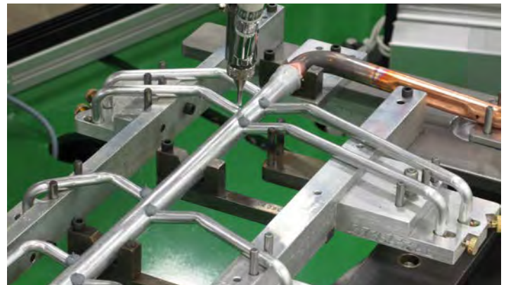
Linear robot guides applicator to dispense multiple deposits of GNC-1070-401 aluminum brazing paste to header joints.
