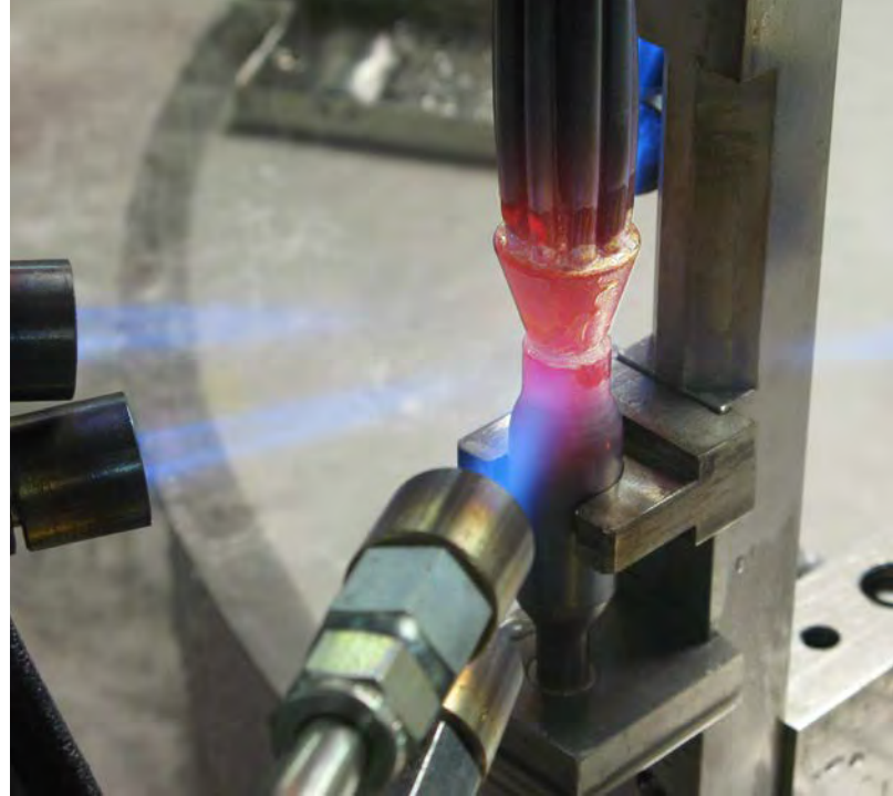
Precision heat pattern distributes filler metal, resulting in void-free joints.
