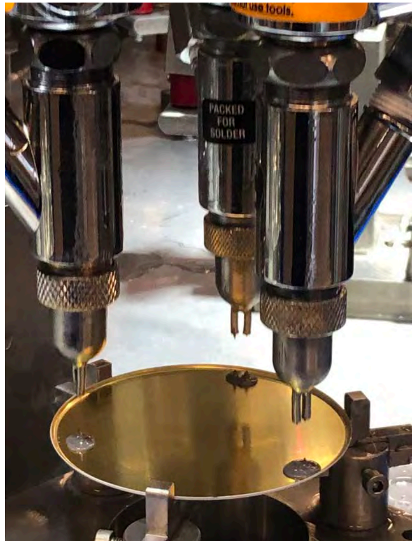
Applicators dispense PAD-136-850 solder paste onto cover plates.
