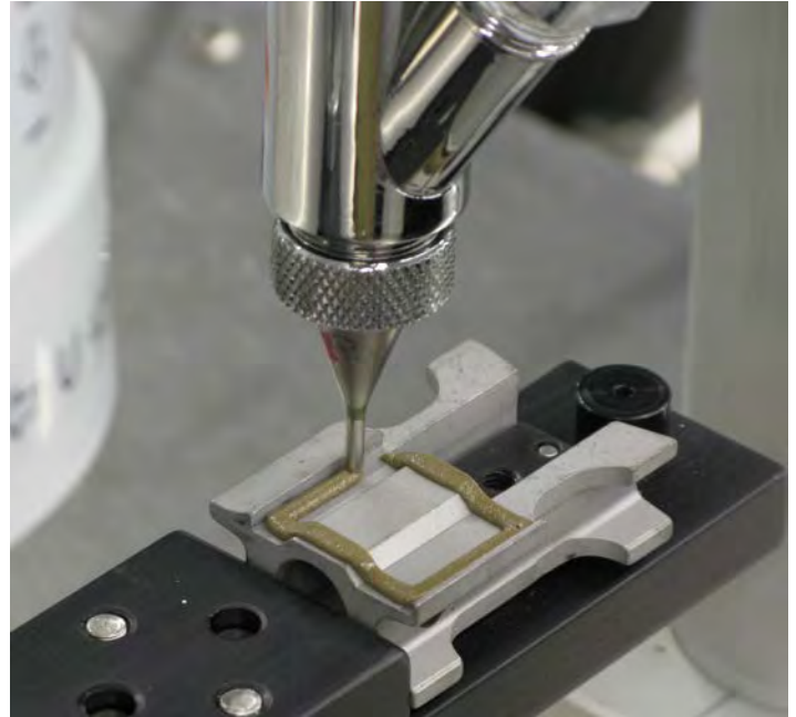
Scara robot moves lower carrier beneath applicator to accept exact pattern of 2MJ-1260-800 braze paste.
